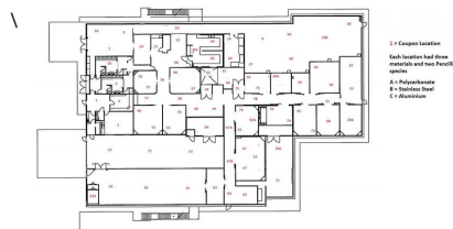
Figure 1: Chemical Indicator locations for each of 240 samples (80 locations x 3 materials; 316L Stainless Steel, Perspex (Acrylic) and Aluminium.
