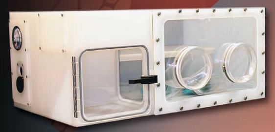
The MINI-Q™ is designed to house small groups of mice in a strict quarantine environment. Glovebox construction is of hight impact resistant polymers which are welded to provide an air tight seal. Acrylic doors feature silicone gaskets and single pull latches. Each glovebox includes HEPA filtered (99.97% at .3 Microns), intake and exhaust with airflow and magnehelic gauge. As shown, stackable units are available with cart for portability.
